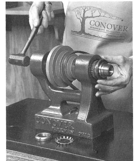
Removal of the headstock spindle. Slight blow from a soft faced mallet coaxes front seal out which technician is now holding.
