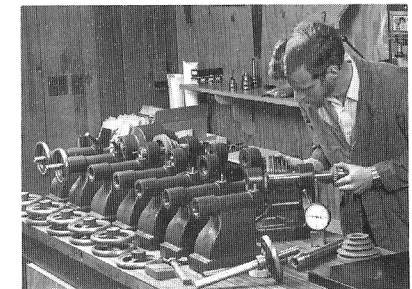
Conover Lathes are hand assembled in small lots. Frequent quality checks during the manufacturing process combined with a dynamic "run in" insure that your lathe is tuned to perfection.
